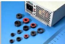
The Magnetic Amplifier (Mag Amp) regulation principle offers a low cost, efficient and, owing to the simple design, highly reliable solution for secondary output regulation in switched-mode power supplies with multiple outputs.
